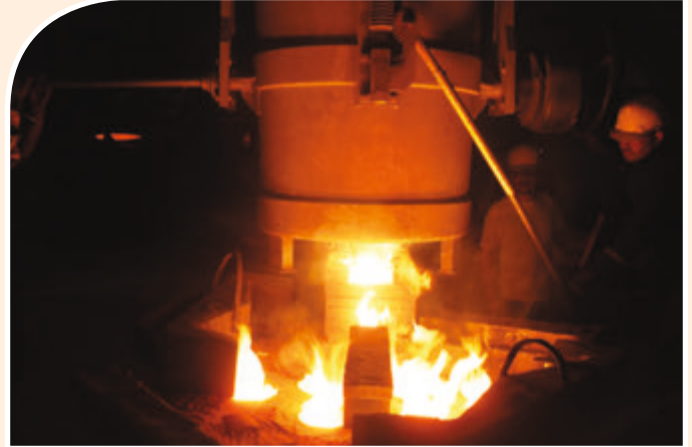
Döküm /Casting Process
